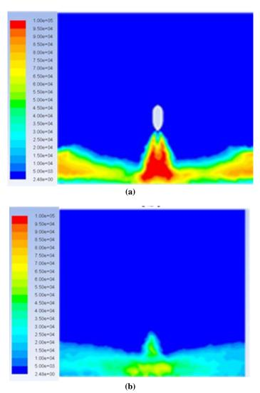
Figure 10. Contour of turbulent viscosity ratio produced during the simulation of case 5: (a) top surface, (b) Bottom surface
