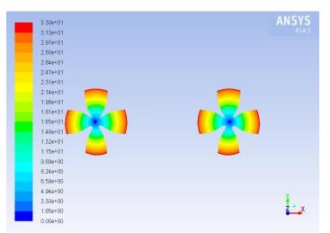
Figure 4. Velocity contours of the propellers
